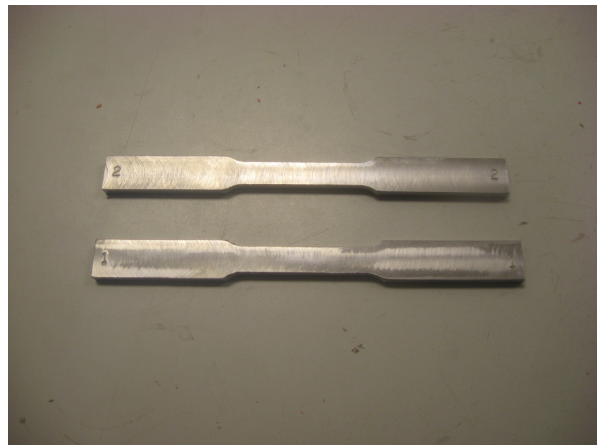
Machined Test Specimens obtained from steel samples No.s 1 and 2.
